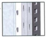
Fit the back-wall into the perforations of the uprights working from the bottom up.
