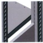
Insert the sides into the slots of the uprights starting at the bottom and following the panel profile.
